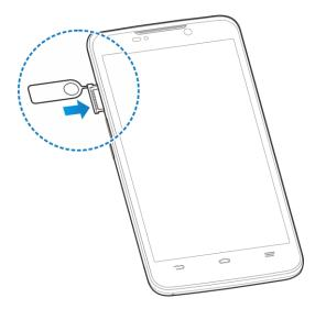
2. Pull out the SD card tray and place the SD card in the tray making sure it is properly oriented. Then carefully install the tray back.
