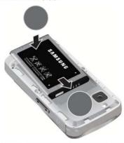
Replace the cover by lining up the tabs and then firmly sliding the cover away from the lens until it snaps into place.
