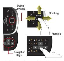
The Optical Joystick acts as a dual touch-sensitive mouse and OK/Enter key. As you navigate through a menu, options are highlighted. Select any option by highlighting it and pressing .
