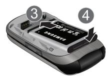
Replace the cover by lining up the tabs and then firmly sliding the cover away from the lens until it snaps into place.
