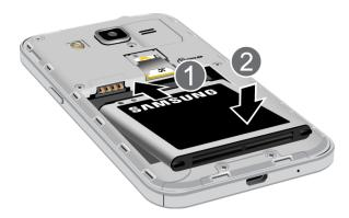
Align the contacts of the battery with the contacts in the phone.
