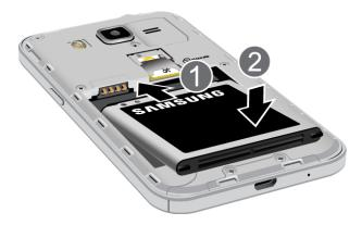
Align the contacts of the battery with the contacts in the phone.
