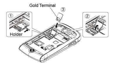
5. Replace the card and card holder and gently press them, and then slide the holder in the direction of arrow to lock it.
