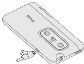
2. Plug the AC adapter in to an electrical outlet to start charging the battery.
